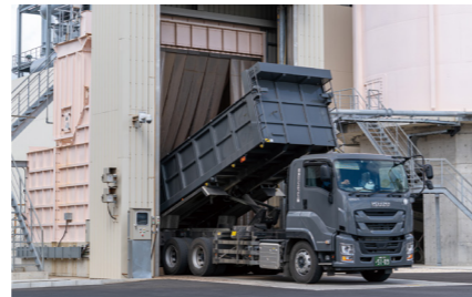
Trucks with a covered cargo bed control dust dispersion during transportation
